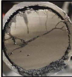
Recovered core showing complexity of hydraulically created fractures
